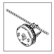
4 Ensure the chain connector is at the back side of the Chain Mech.
